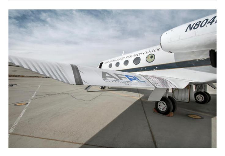
If you've ever sat over the wing of a plane, you've seen the robotic motion of the wing flaps as they adjust to conditions during landing and takeoff. These flaps—along with the landing gear—are a primary source of noise and drag because of the gaps between them. (Engines have actually quieted down dramatically since the 1960s and 1970s, **Collier** explains.) A single long wing flap that could still move and adapt would not only make flying more efficient, it would make it much quieter.
