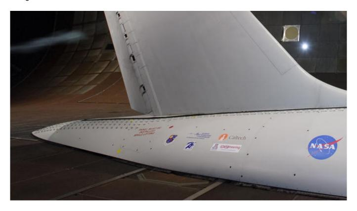
In some cases, the huge scale of these **design**s require extensive planning just to test. Like one full-scale Boeing 757 tail section which, at almost 30 feet tall, required <u>months of planning</u> to install inside a cavernous **NASA** wind tunnel, currently the largest in the world.
