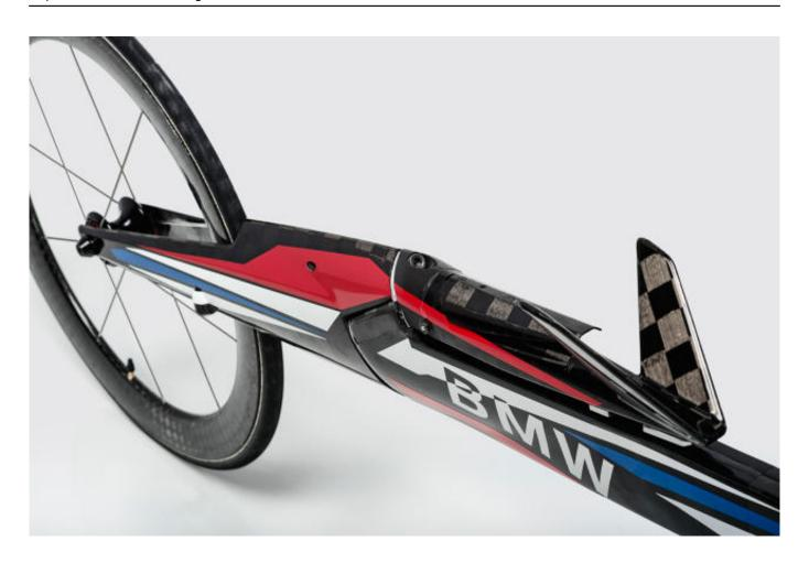
First, the **design** team scanned one of the athletes in 3-D, sitting in his chair. From there, **BMW** built a computer model that could simulate changes in aerodynamics. The designers learned that about 50% of aerodynamics can't be altered, because the drag comes from the racer's body. But by making various tweaks—small, angular changes to the frame that the firm avoids going into detail about—they were able to shave off 15% of the drag.
